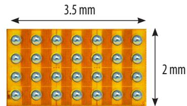
Figure 1: EPC2053 100 V eGaN FET with 4 mΩ on-resistance
