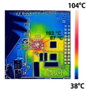
Figure 5: Thermal image of the EPC9093 operating at 500 kHz, 12 V and 20 A with 400 LFM airflow
