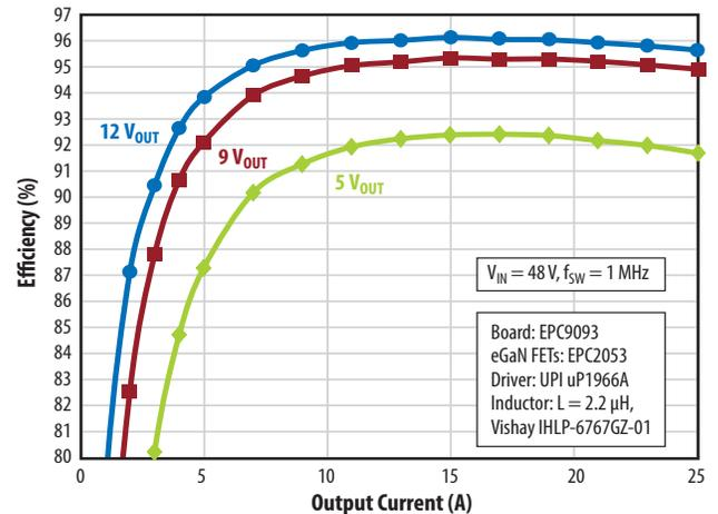
Figure 6: EPC9093 efficiency vs. output current for 48 V<sub>IN</sub> to 5, 9 and 12 V<sub>OUT</sub> when operating at 1 MHz and using EPC2053 eGaN FETs
