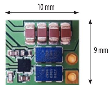
Figure 3: The EPC9093 development board fitted with EPC2053
