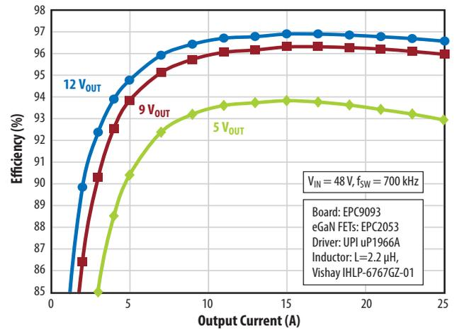
Figure 4: EPC9093 efficiency vs. output current for 48 V<sub>IN</sub> to 12 V<sub>OUT</sub> when operating at 700 kHz and using EPC2053 eGaN FETs
